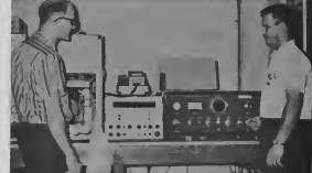
PETE SCHERMERHORN and Felix Croes (r) check operation of new temperature programmed gas chromatograph, coupled to electronic integrator and printing machine.
